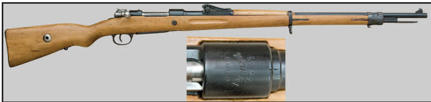
Fig. 4 Czech VZ-98 rifle assembled at Zbrojovka, Brno from German parts. The barrel and many other parts bear German inspection marks. (Author's collection.)
